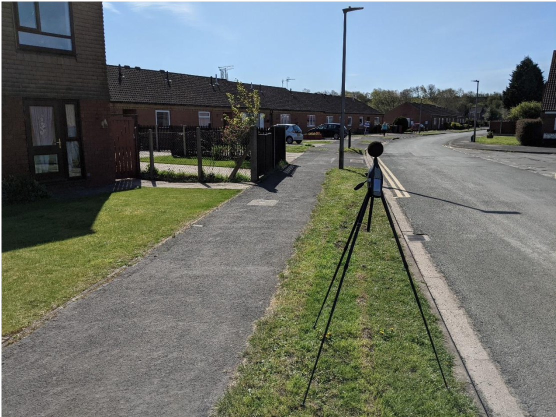
Figure 27: R9 Bolsover Road Noise Monitoring Setup
