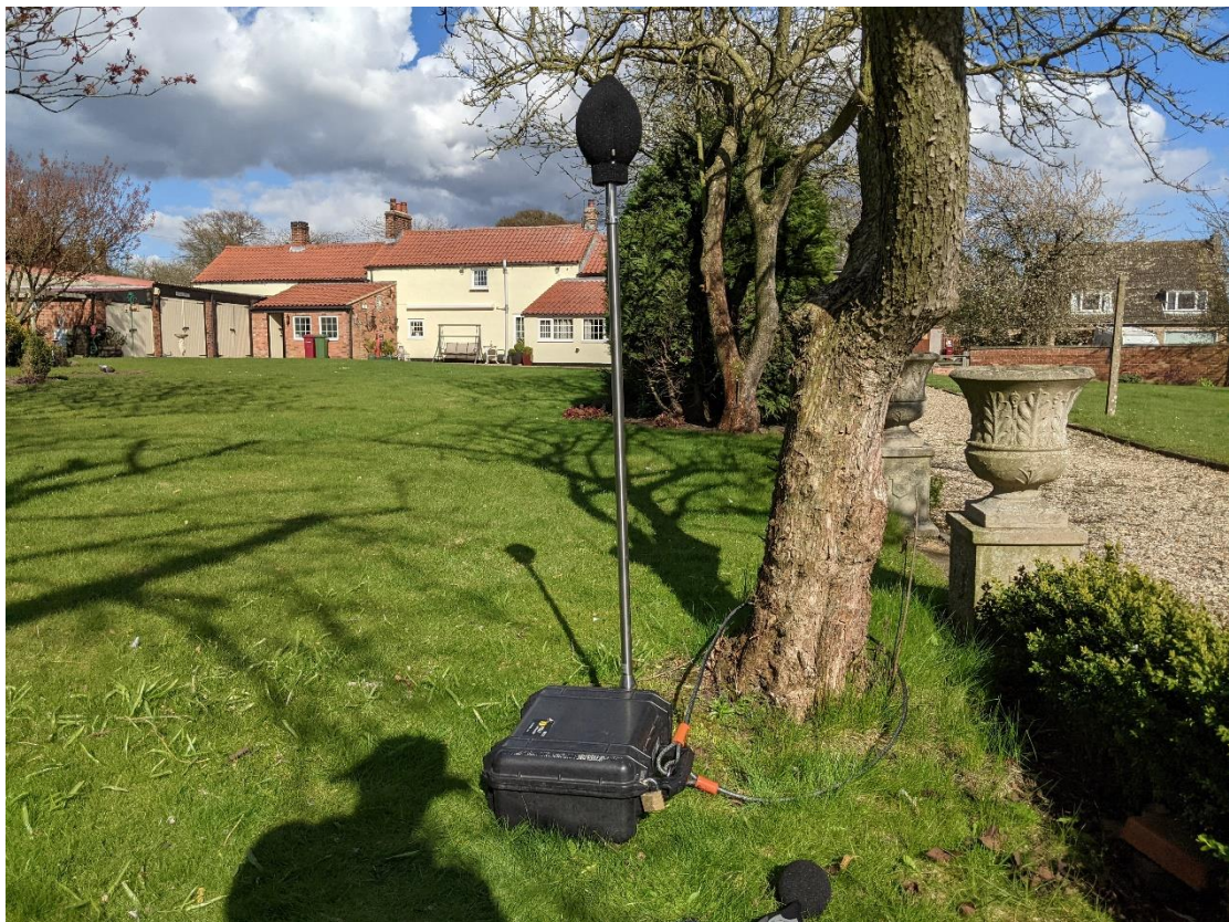
Figure 7: Noise Monitoring Setup at the Forge, Flixborough
